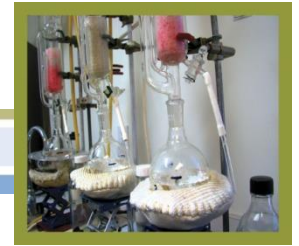
Soxhlet Extractors used for Fat & Oil
